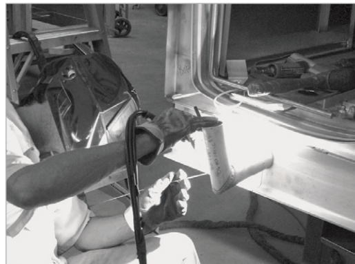
ASME, Section IX Qualified Welder Working on a Bag-in/ Bag-out Filter Housing
